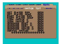
Pressing an action button while SWITCH TEST is highlighted will execute the switch test mode. The highlight will descend to the switch test box, and any previous PASSED flags will be cleared. Pressing and then releasing a switch will cause a PASSED to appear by that switch, as it has now been seen in both the OPEN and CLOSED states. You must pass all player switches (those displayed without parentheses around them in the switch list) to exit the switch test and return to the TESTS menu.
